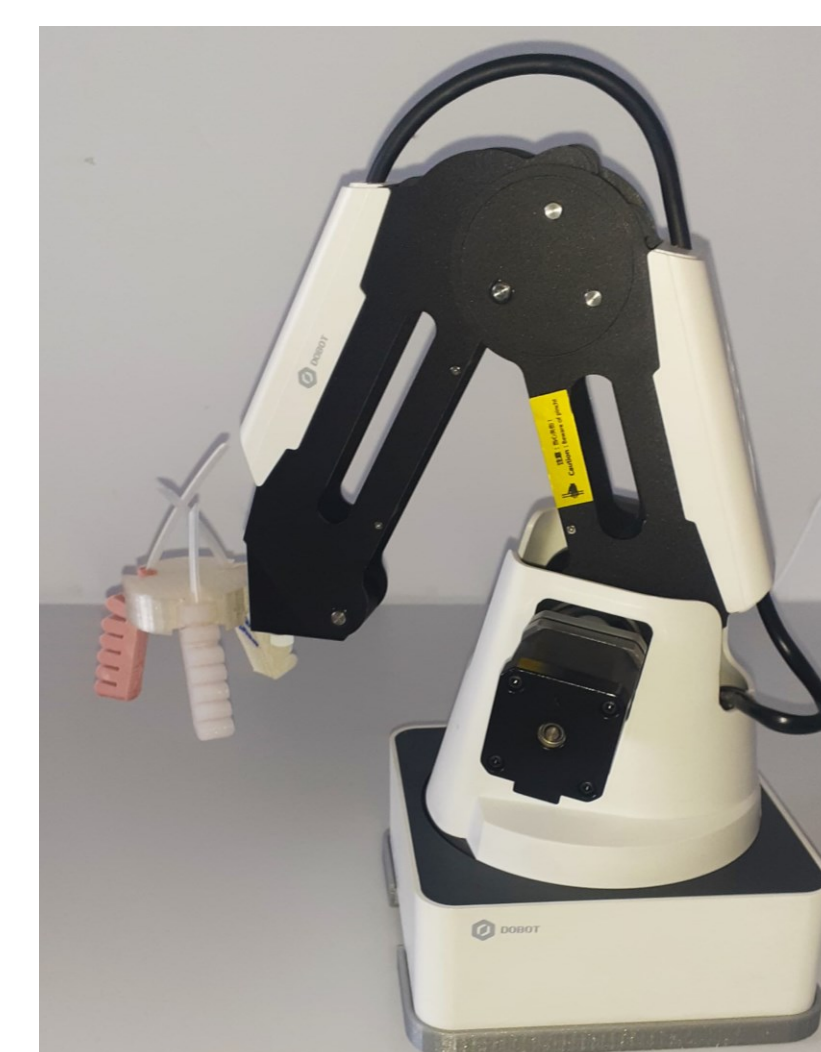
Figure 8: Dobot with Grippers made of Filaflex and Elastosil M4601 A/B, DragonSkin Fast 10 silicones.
